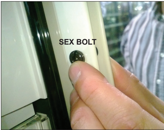
Fig. 7 Sex bolts for closing case frame gap
