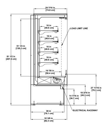
Please consult Hillphoenix Engineering Reference Manual for dimensions, plan views and technical specifications. Specifications subject to change without notice. Designed for optimal performance in store environments where temperature and humidity do not exceed 75°F and 55% R.H. Certified to UL 471. NSF Standard 7 and CAN/CSA C22.2.
